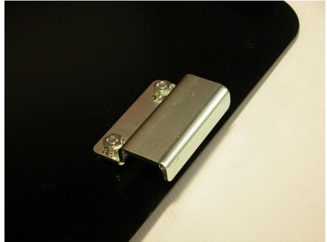
**Step 3:** Lift the engine skid plate and place the skid plate clamp over the forward lip of the factory transfer case skid plate. Then rotate the engine skid plate into position and slide it over the threaded portion of the lower control arm bolt that you reversed in the first step.
