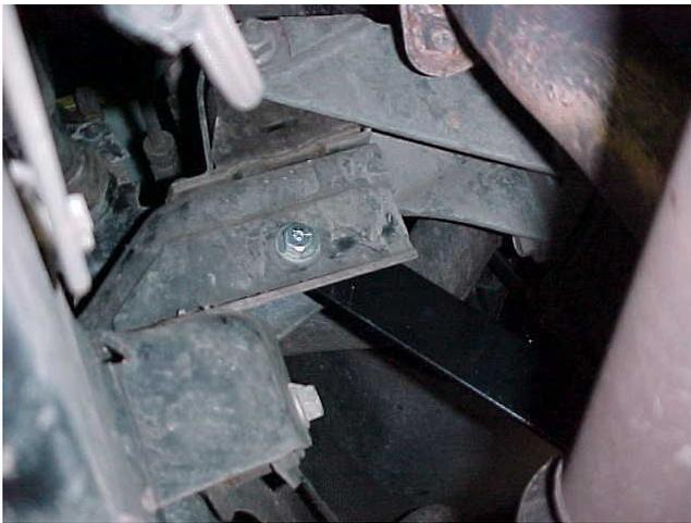
**Step 5:** Take the strut rod and attach it between the motor mount and the skid plate. Use one 3/8-16 bolt, lock washer, and nut to bolt it to the front of the skid plate and use the remaining 1/2-13 bolt, washer and nut to attach it to the rear of the motor mount. The view in the photo is from the rear on the driver's side.
