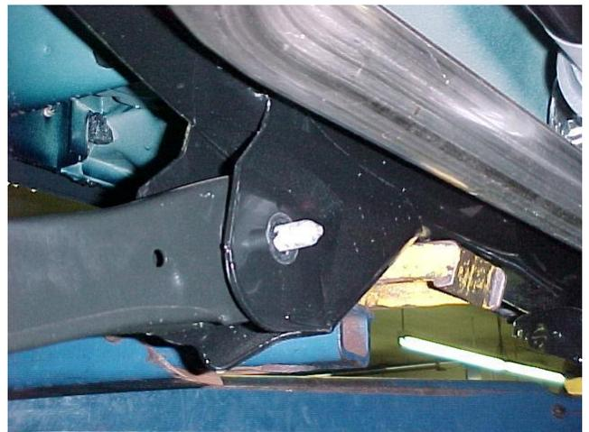
**Step 2:** Take the engine skid plate and loosely attach the transfer case skid plate clamp using two 3/8-16 bolts with lock washers. Be sure that the hook portion of the clamp is facing the rear edge of the skid plate as show at right.
