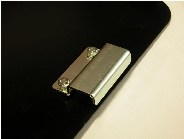
**Step 4:** Take the engine skid plate and loosely attach the transfer case skid plate clamp using two 3/8-16 bolts with lock washers. Be sure that the hook shaped portion of the clamp is facing the back of the skid plate as shown above.
