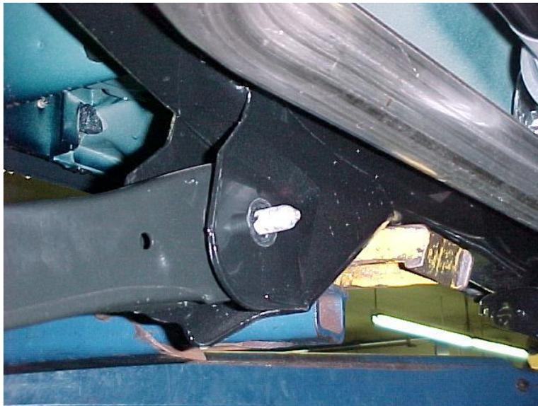
**Step 2:** Take the T-shaped nut plate and slide it into the driver's side motor mount through the top opening. Once the nuts can be seen through the two holes in the lower side of the motor mount, the tab may be folded over to hold the nuts in position. It is helpful to give the tab a slight arch before inserting it into the motor mount.
