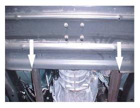
**Step 3:** Lift the engine skid plate and slide it over the threaded portion of the lower control arm bolt. Position the rear edge of the engine skid plate within the notched out area on the factory transfer case skid plate as indicated by the arrows in the picture to the left.
