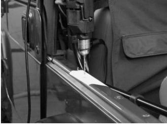
**Step 4:** Take a mounting bracket and place it in position on the tub centered around the mark you made in Step 3. Then mark the holes making sure that they are centered on the top lip of the tub.
