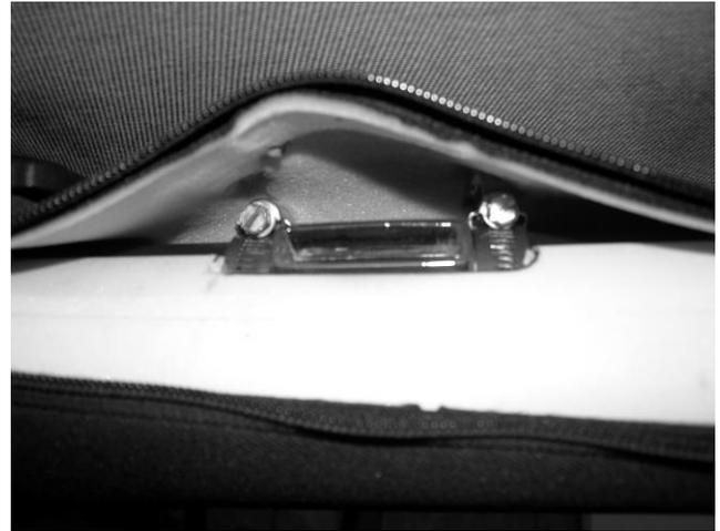
**Step 4:** Reinstall the fabric covers and using a razor blade, make an opening through the material to allow the slat to slide into the bow socket.
