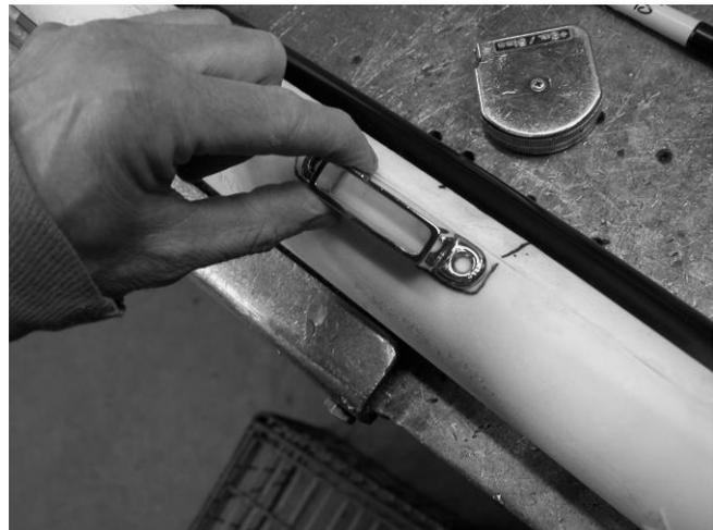
**Step 1:** Remove the fabric cover from the roll bar tube that extends forward above the door. Mark the location on the padding where you want to place the Top Prop. It should be roughly centered above the door. Then remove the foam padding from the tube being careful not to break the foam. There are plastic fasteners along the bottom of the padding that you simply pull out of holes in the roll bar tubing.
