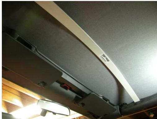
**Installing the Slat:** Simply insert one end of the slat into one of the bow sockets, push the slat up in the middle, and insert the other end of the slat into the other bow socket. That's all there is to it!
