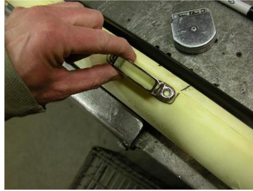
**Step 3:** Place a bow socket along the top edge of the padding, centered on your mark, and draw a line around it as shown above left. Then place the socket along the line you just drew and draw a second line around the socket as shown in the photo above right. Then cut away the padding material along the lines just made.
