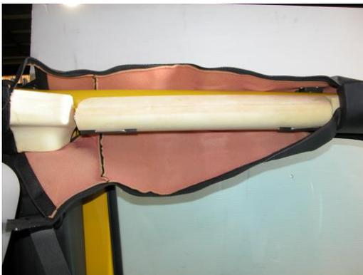
**Front Top Prop Step 1:** Open the fabric cover from the roll bar tube above the door as show above left. The zipper starts at the rear of the bar, near the main roll bar hoop.
