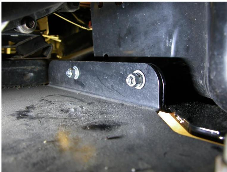
**Step 9:** Re-install the factory mounting bolt for the transfer case skid plate through the gas tank skid plate. The 1/2" thick aluminum spacer is used between the gas tank skid and the mounting bracket of the transfer case skid plate.
