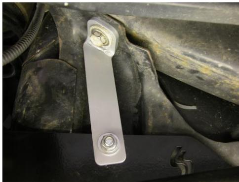
**Step 8:** If using our Skid Row Offroad transfer case skid plate, use the remaining two carriage head bolts, flat washers, lock washers, and nuts to attach the gas tank skid plate to the transfer case skid plate as shown below.
