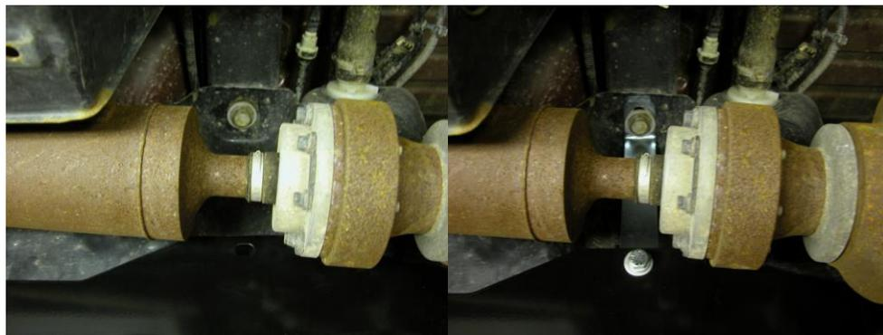
**Step 7:** The Mounting Bracket w/o Nut is installed at the rear, outboard side of the skid plate, near the Skid Row logo. Again, remove the factory skid plate mounting bolt from the chassis. Then remove the nut that was installed on the carriage bolt. Place the bracket over the carriage bolt and install the flat washer, lock washer, and nut. Then re-install the factory mounting bolt through the bracket as shown.
